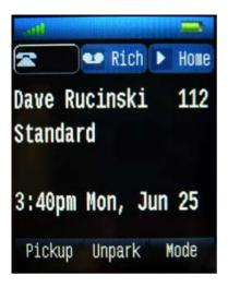
Push the right direction of the 4-way controller twice to highlight the Speed Dial button appearance labeled "Home."
