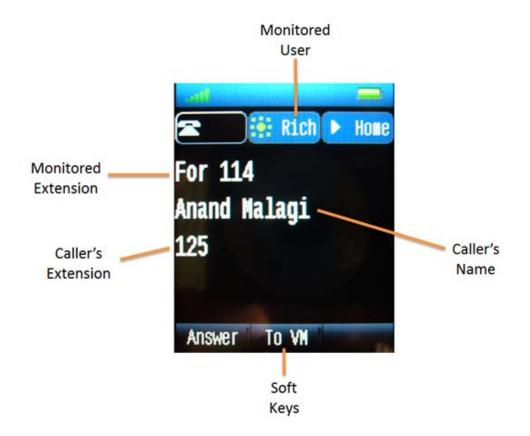
You can pick up the call while it is ringing by first highlighting and then selecting the monitored extension using the 4-way controller (or by pressing the **Answer** soft key). You can send the call to the monitored extension's voicemail by pressing **To VM**. You can also answer a call after the owner of the monitored extension has put it on hold by pressing the **Pickup** soft key.
